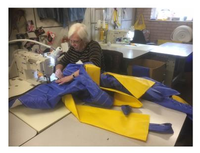
That afternoon, three skilled machinists from PLCS's sewing room worked in tandem to expedite the manufacturing process, cutting and sewing the various elements of the polyurethane-coated nylon mould, which was completed and quality-approved on the same day.
