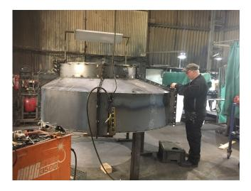
The proximity of multiple utilities around the valve resulted in the mold being constructed in six different segments which would allow each piece to be inserted into the excavation between the cables.
